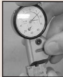
2. Tilt the gage from side to side to locate the shortest depth location. Then, turn the indicator dial to align the needle with zero.
