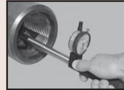
2. Position the contact point in the root of the thread.
