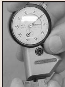
3. Tighten the indicator clamp and remove the gage from the standard. Remember to recheck the zero position.
