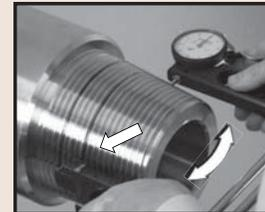
6. Use the lower arm as a pivot, sweep the upper contact point side to side to locate the largest indicator reading.
