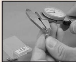
2. Using calipers, verify the size of the contact point.
