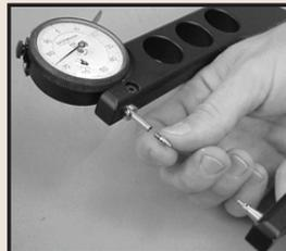
4. To secure the contact points, open a paper clip and insert it into the hole in the contact point's shaft. Rotate, using moderate pressure, to tighten the contact point.
