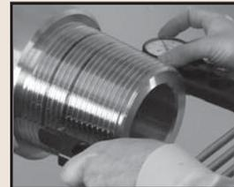
8. Remove the gage from the first marked thread and insert into the second marked thread.
