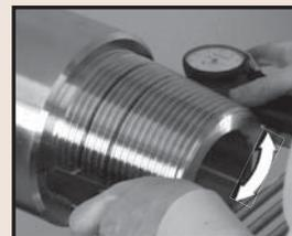
9. Use the lower arm as a pivot, sweep the upper contact point side to side to locate the largest indicator reading.
