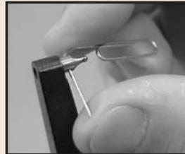
**\*Do Not** use pliers to tighten the contact points, as damage may result.
