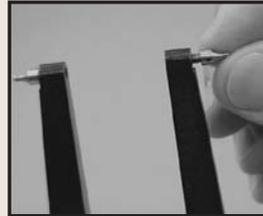
4. To secure the contact points, open a paper clip and insert it into the hole in the contact point's shaft. Rotate, using moderate pressure, to tighten the contact point.
