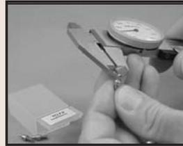
2. Using calipers, verify the size of the contact point.
