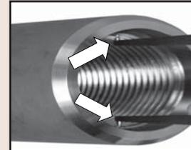
5. Adjust the location of the lower arm so that the upper arm and contact point are seated in the same marked thread of the part.
