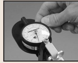
7. Turn the indicator dial on the IT-6000 gage to align the needle with zero.
