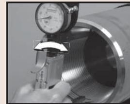
6. While holding the fixed ball contact at the marked location, sweep the upper contact point side to side to locate the largest indicator reading.
