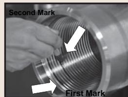
2. Mark another full revolution on the threads of the part one inch back from the first mark. For example, for a 8 pitch thread, count back 8 threads from where you first marked, and mark.
