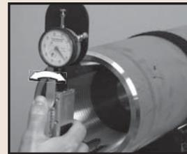
9. Repeat step 4 and place the movable ball contact into the second marked thread.
