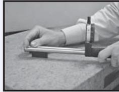
2. Turn the indicator dial to align the needle with zero.
