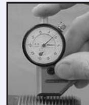
2. Push down on the gage until the gage body rests on the crests of the thread.
