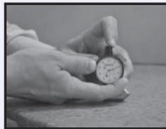
3. Tighten the indicator Bezel clamp.
