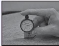
2. Tilt the gage from side to side to locate the shortest depth location. Then, turn the indicator Bezel to align the needle with zero.
