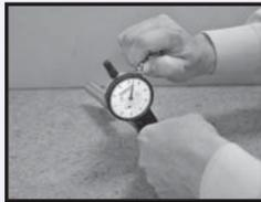
3. Tighten the indicator Bezel clamp.
