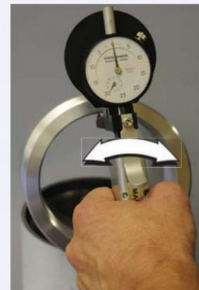
*Note:* Be sure that the small revolution counter on the indicator is pointing to the same number as when the gage was zeroed.
