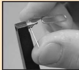
4. To secure the contact points, open a paper clip and insert it into the hole in the contact point's shaft. Rotate, using moderate pressure, to tighten the contact point.
