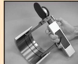
10. Using the lower arm as a pivot, sweep the upper contact point side to side to locate the largest indicator reading.
