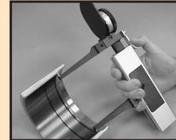
6. While holding the fixed ball contact at the marked location, sweep the upper contact point side to side to locate the largest indicator reading.
