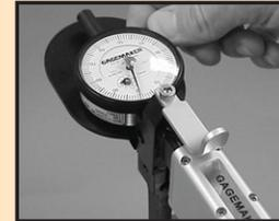
7. Turn the indicator dial on the IT-6000 gage to align the needle with zero.
