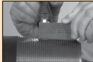
5. Holding the template lightly in your hand, slide it counter clockwise around the connection. If there is any debris in the groove it will stop the template. Remove all debris from the thread groove and re-check. This is a major cause of thread damage to made-up connections.
