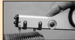
2. Tilt the gage forward to seat the moveable contact point into the thread.
