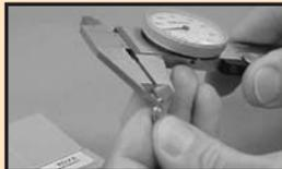
3. Install one contact point into the moveable point holder at the front of the gage.
