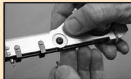
6. Once installed, insert a paper clip into the hole in each contact point and tighten.
