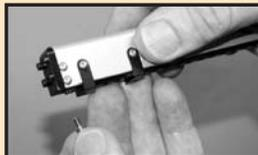
4. Determine the location for the other contact point based on the interval of lead required for the inspection. The increments in the lead gage are set at ¼" intervals from 1" – 4".
