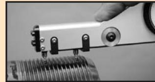
3. Apply pressure to the nose of the gage with the index finger. Do not apply excessive force to the gage, just enough to keep the moveable point in contact with the thread flanks. Then, using the rear contact point as the pivot point, sweep the gage to locate the shortest distance.
