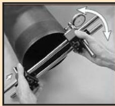
**Note:** Be sure that the small revolution counter on the indicator is pointing to the same number as when the gage was zeroed.
