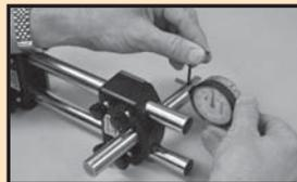
4. Thread each pivot shoe into the upper and lower arms of the gage.
