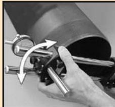
4. Rotate the gage 90 degrees and sweep for the largest reading again. If your second reading is greater or less than the first, sweep 180° around the part to find the largest and smallest values.
