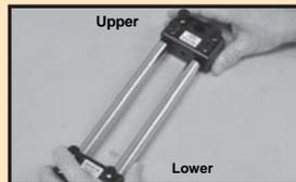
2. Insert the arms into the upper and lower blocks. Be sure the upper and lower arms are positioned properly, as shown, before continuing with the gage setup.
