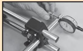
5. Align each pivot shoe parallel with the groove on each arm.
