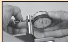
6. Tighten the binder nut to secure. Be careful not to over-tighten the binder nut, which may cause damage to the indicator.
